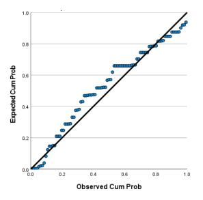
*Note.* Normal p-p plot of regression standardized residual showing an approximately normal distribution of residuals. "The P-P plot of the residuals is the preferred graphical tests for normality" (Flatt & Jacobs, 2019, p. 488).
